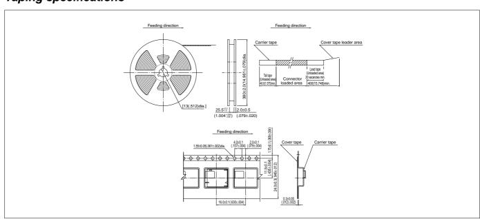
Note: 1. Conforms to JIS C0806. Tape width and tape connector recess dimensions depend the connector outer dimensions.
