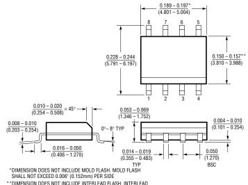
\*\*DIMENSION DOES NOT INCLUDE INTERLEAD FLASH. INTERLEAD FLASH SHALL NOT EXCEED 0.010" (0.254mm) PER SIDE
