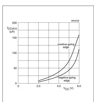
Fig.14 Average  $I_{CC}$  for HC1G Schmitt-trigger devices; linear change of V<sub>I</sub> between  $0.1V_{CC}$  to  $0.9V_{CC}$ .
