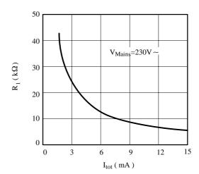
Figure 7. Maximum resistance of R<sub>1</sub>
