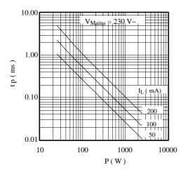
Figure 5. Output pulse width
