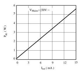
Figure 8. Power dissipation of  $R_1$  according to current consumption
