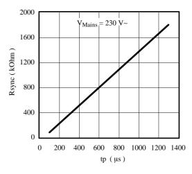
Figure 6. Synchronization resistance
