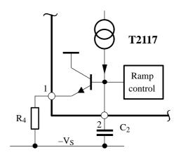
Figure 3. Pin 1 internal network
