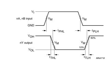
For 74HC2G02:  $V_M$  = 50%;  $V_I$  = GND to  $V_{CC}$ . For 74HCT2G02:  $V_M$  = 1.3 V;  $V_I$  = GND to 3.0 V.
