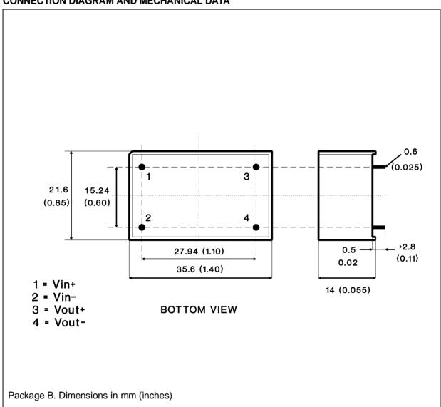
CONNECTION DIAGRAM AND MECHANICAL DATA
