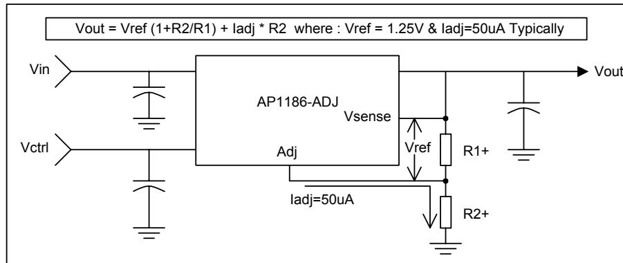
The AP1186-ADJ keeps a constant 1.25V between the Vsense pin and the Adj pin. By placing a resistor R1 across these two pins and connecting the Vsense and Vout pin together, a constant current flows through R1, adding to the Iadj current and into the R2 resistor producing a voltage equal to the  $(1.25/R1)*R2 + Iadj*R2$ . This voltage is then added to the 1.25V to set the output voltage. This is summarized in the above equation.
