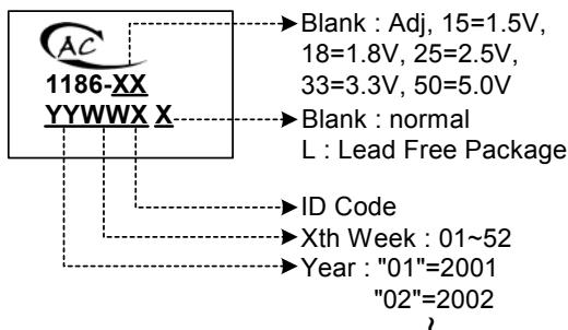
**1.5A Ultra Low Dropout Positive Adjustable or Fixed-mode Regulator****■ Package Information**
