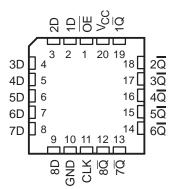
OE does not affect internal operations of the latches. Old data can be retained or new data can be entered while the outputs are in the high-impedance state.
