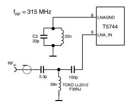
Please note that for all coupling conditions (see Figure 5 and Figure 6), the bond wire inductivity of the LNA ground is compensated. C3 forms a series resonance circuit together with the bond wire. L = 25 nH is a feed inductor to establish a DC path. Its value is not critical but must be large enough not to detune the series resonance circuit. For cost reduction, this inductor can be easily printed on the PCB. This configuration improves the sensitivity of the receiver by about 1 dB to 2 dB.
