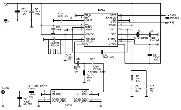
Figure 17. Application Circuit:  $f_{RF} = 315 \text{ MHz}$ , with SAW Filter
