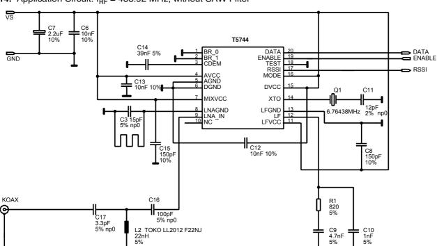
**Figure 14.** Application Circuit:  $f_{RF} = 433.92$  MHz, without SAW Filter
