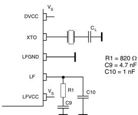
The passive loop filter connected to Pin LF is designed for a loop bandwidth of BLoop = 100 kHz. This value for BLoop exhibits the best possible noise performance of the LO. Figure 4 shows the appropriate loop filter components to achieve the desired loop bandwidth
