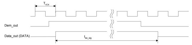
Figure 13. Debouncing of the Demodulator Output
