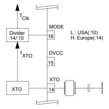
Pin MODE can now be set in accordance with the desired clock cycle  $T_{Clk}$ .  $T_{Clk}$  controls the following application-relevant parameters:
