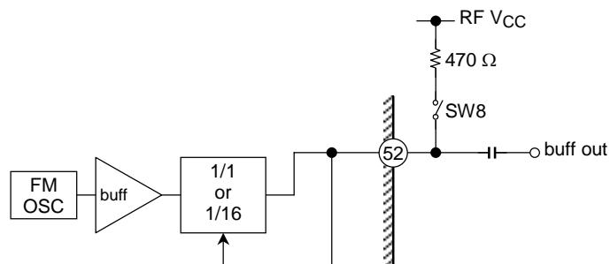
Divider of FM OSC ON/OFF switching is controlled by external pull-up resistor of pin 52.
