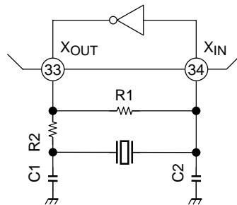
A Daishinku K.K. crystal oscillator (with a maximum CI value of 30 kΩ) was tested with Toshiba's test PCB (using capacitors of 18 pF and 22 pF).
