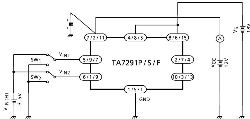
(Note) HEAT FIN of TA7291F is connected to GND.
