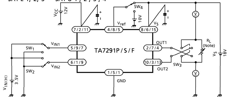
(Note)  $I_{OUT}$  calibration is required to adjust specified values of test conditions by  $R_L$ .
