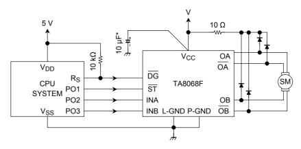
\*: Connect this capacitor as close to the IC as possible
