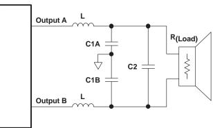
Figure 10. Demodulation Filter
