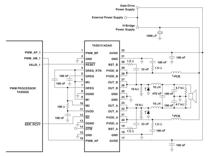
L<sub>PCB</sub>: TRACK IN THE PCB (1 mm wide and 50 mm long)
