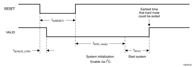
NOTE: RESET must be asserted low at least 100  $\mu s$  after DVDD reaches 3.0 V.
