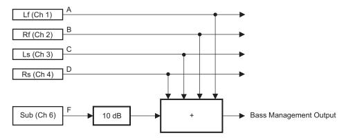
Bass Management Output = BS\_Out (linear) = Ch 6 =  $F \times 3.121 + (A + B + C + D)$ BS\_Out (log) =  $20 \times log$  (BS\_Out)
