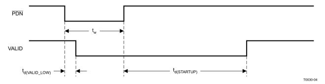
Figure 6. Power-Down Timing
