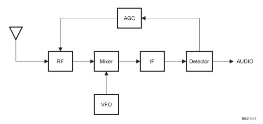
Figure 45. AM Receiver Architecture
