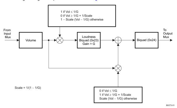
Figure 46. Biquad Gain Control Structure
