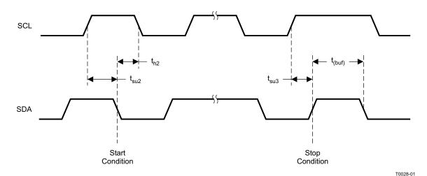
Figure 4. Start and Stop Conditions Timing
