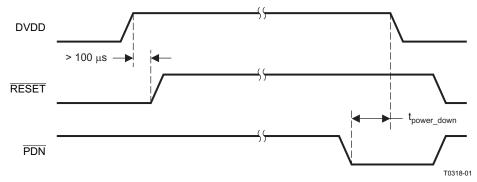
NOTE:  $t_{power\_down}$  = time to wait before powering down the supplies after  $\overline{PDN}$  assertion = 725  $\mu s$  + power-stage stop time defined by register 0x1A
