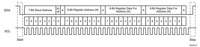
Figure 37. Typical I<sup>2</sup>C Sequence
