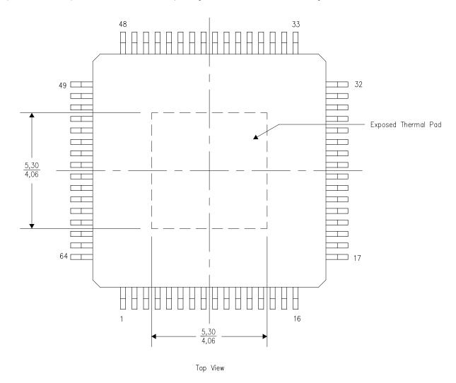
NOTE: All linear dimensions are in millimeters
