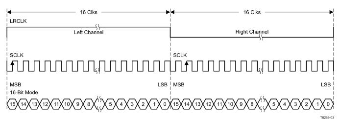
Figure 36. Right-Justified 32-f<sub>S</sub> Format
