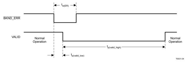
**Figure 9. Error Recovery Timing**
