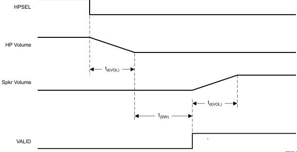
Figure 12. HPSEL Timing for Headphone Extraction
