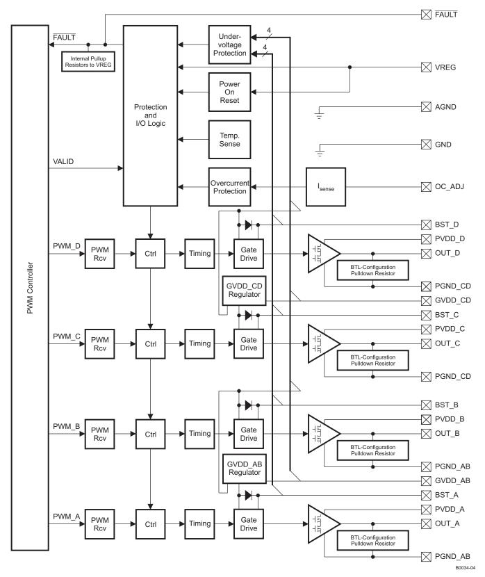
Figure 1. Power Stage Functional Block Diagram
