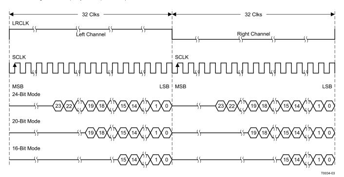
Figure 34. Right-Justified 64-f<sub>S</sub> Format
