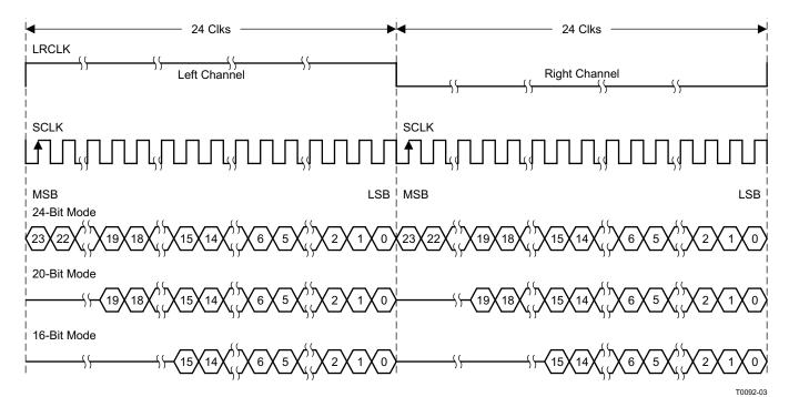
Figure 35. Right-Justified 48-f<sub>S</sub> Format
