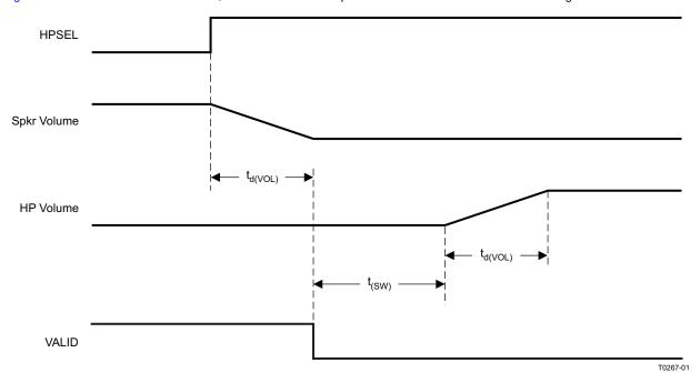
Figure 11. HPSEL Timing for Headphone Insertion
