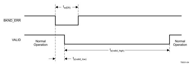
Figure 6. Error Recovery Timing
