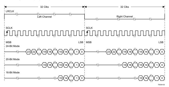
Figure 36. Right Justified 64-f<sub>S</sub> Format
