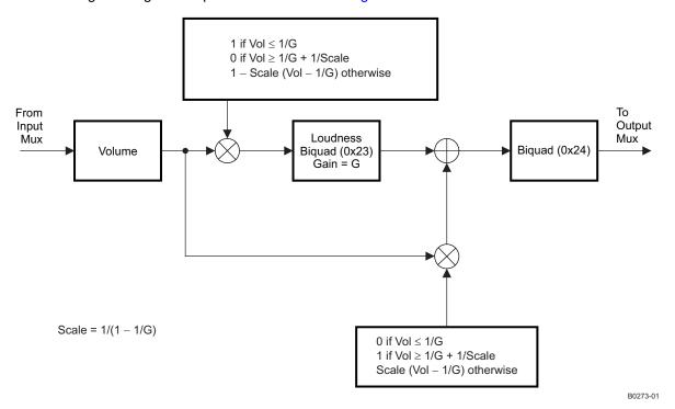
Figure 46. Biquad Gain Control Structure
