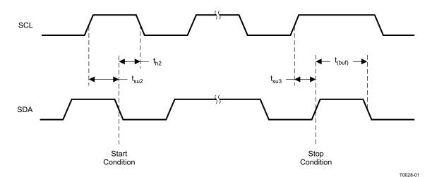
Figure 3. Start and Stop Conditions Timing
