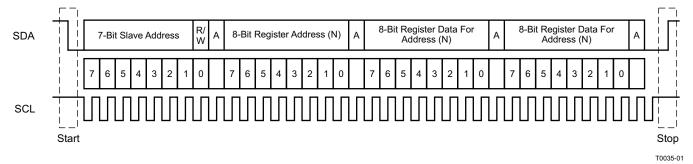
Figure 39. Typical I<sup>2</sup>C Sequence
