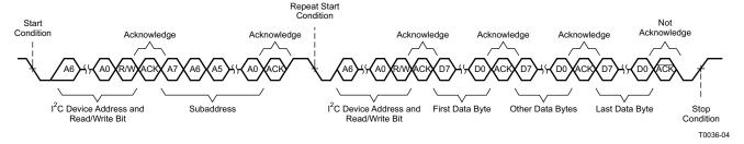
Figure 43. Multiple Byte Read Transfer
