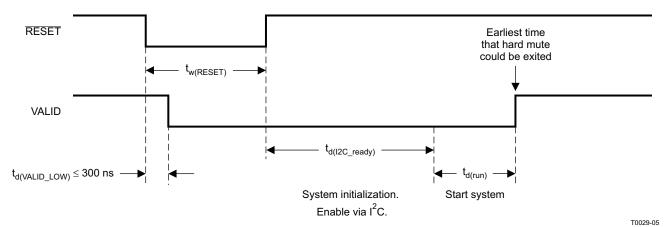
Figure 4. Reset Timing
