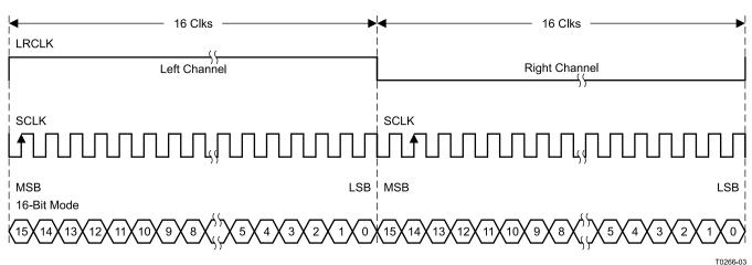
Figure 38. Right Justified 32-f<sub>S</sub> Format
