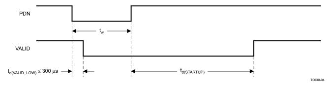
Figure 5. Power-Down Timing
