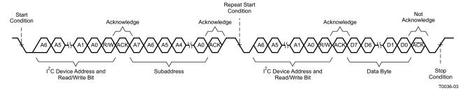
Figure 42. Single-Byte Read Transfer
