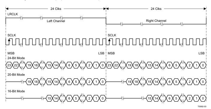
Figure 37. Right Justified 48-f<sub>S</sub> Format
