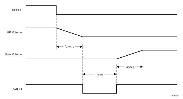
Figure 9. HPSEL Timing for Headphone Extraction
