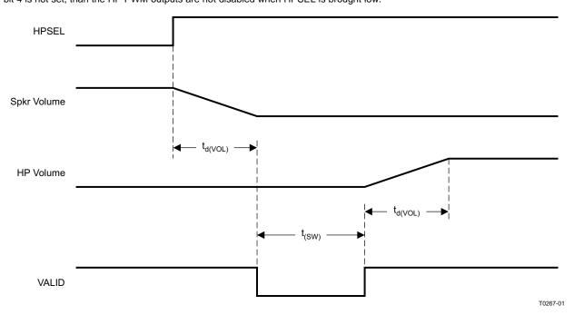
Figure 8. HPSEL Timing for Headphone Insertion
