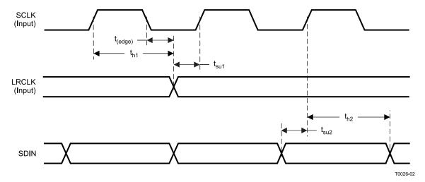
Figure 1. Slave Mode Serial Data Interface Timing
