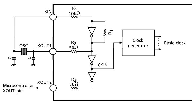
Recommended oscillators : 8MHz : Murata 8MHz Ceralock ceramic oscillator (CST8, 0MTW)
