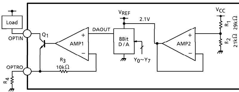
(Note) Because the AMP1 output is held low when the D/A data are 00H, Q1 is OFF.
