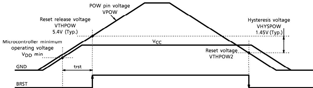
The above chart shows the recommended design for the relationship between the mains power monitoring voltage (VPOW) and the system power supply (VCC).
