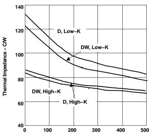
Figure 10. Thermal Impedance vs Air Flow
