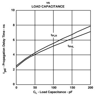
A. NOTE: This graph is included as an aid to the system designers. Total circuit delay varies with load capacitance. The total delay is the sum of the delay due to external capacitance and the intrinsic delay of the device. Intrinsic delay is listed in the table above as the 0 pF load condition. The incremental increase in delay between the 0 pF load condition and the actual total load capacitance represents the extrinsic, or external delay contributed by the load.
