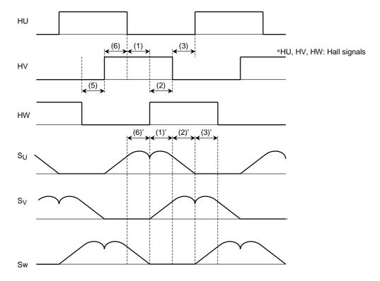
In the above diagram, the modulation waveform (1)' data moves forward by the 1/32 time width of the time (1) from HU:  $\uparrow$  to HW:  $\downarrow$ . Similarly, data (2)' moves forward by the 1/32 time width of the time (2) from HW:  $\downarrow$  to HV:  $\uparrow$ .
