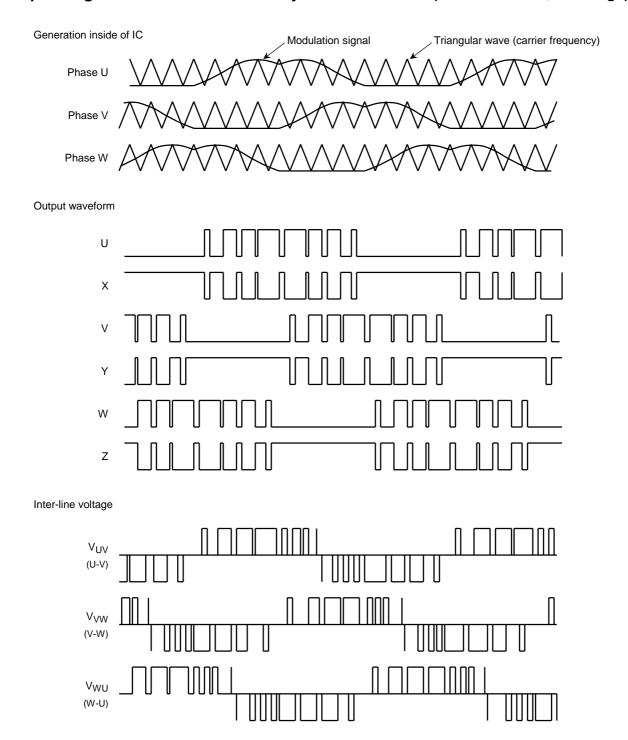
When the motor is driven by a sine wave, the motor is accelerated/decelerated according to the On duty of TONU when the amplitude of the modulation symbol changes by voltage  $V_e$  (see the diagram of output On duty on page 11).
