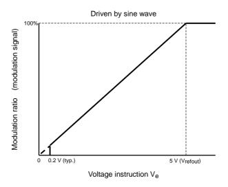
The modulation waveform is generated using Hall signals. Then, the modulation waveform is compared with the triangular wave and a sine-wave PWM signal is generated.
