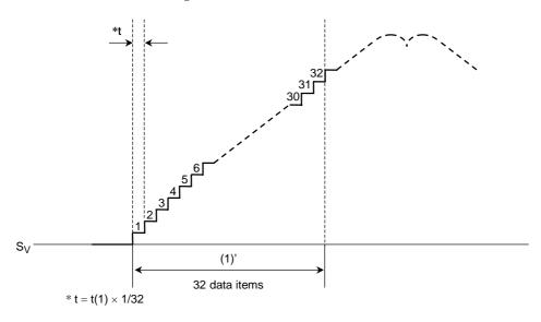
The modulation wave is brought into phase with every zero-cross point of the Hall signal.
