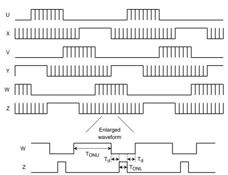
To stabilize the bootstrap voltage, the lower outputs  $(X,\,Y,\,\text{and}\,Z)$  are always turned on at the carrier cycle even during off time. At that time, the upper outputs  $(U,\,V,\,\text{and}\,W)$  are assigned dead time and turned off at the timing when the lower outputs are turned on.  $(T_d\,\text{varies}\,\text{with}\,\text{input}\,V_e)$
