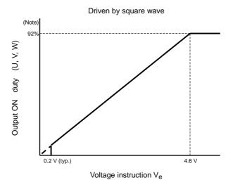
Note: Output ON time is decreased by the dead time. (carrier frequency  $\times$  92% – T<sub>d</sub>  $\times$  2)
