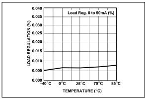
FIGURE 2-3: Load Regulation vs. Temperature. (TC1188)
