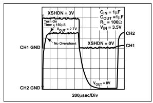
FIGURE 2-9: TC1189 Shutdown Transient Response.
