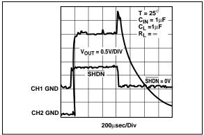
FIGURE 2-8: TC1189 Shutdown Transient Response.
