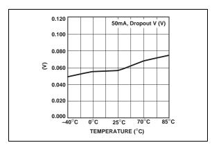
FIGURE 2-5: Dropout Voltage vs. Temperature. (TC1188)
