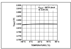
FIGURE 2-2: Output Voltage vs. Temperature. (TC1188)
