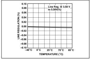
FIGURE 2-1: Line Regulation vs. Temperature. (TC1188)
