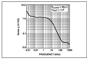
FIGURE 2-6: Output Noise vs. Frequency. (TC1188)
