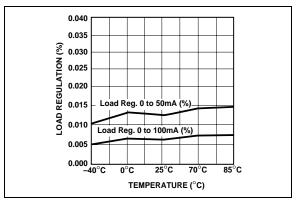
FIGURE 2-4: Load Regulation vs. Temperature. (TC1188)
