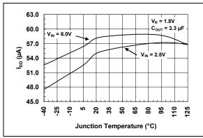
**FIGURE 2-1:** Supply Current vs. Junction Temperature.
