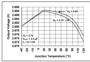
**FIGURE 2-9:** Output Voltage vs. Junction Temperature (0.1 mA).
