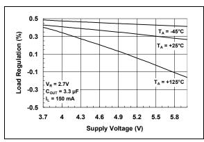
FIGURE 2-8: Load Regulation vs. Supply Voltage.
