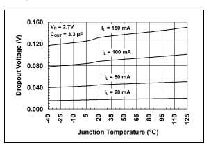
**FIGURE 2-12:** Dropout Voltage vs. Junction Temperature.
