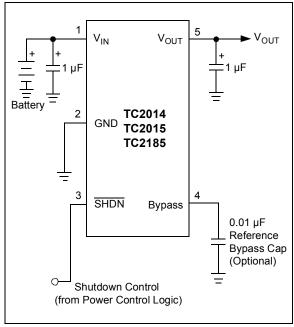
FIGURE 4-1: Typical Application Circuit.
