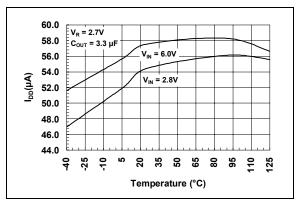
**FIGURE 2-7:** Supply Current vs. Junction Temperature.
