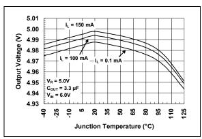
**FIGURE 2-14:** Output Voltage vs. Junction Temperature (150 mA).
