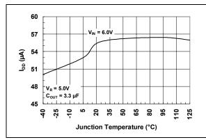
**FIGURE 2-13:** Supply Current vs. Junction Temperature.
