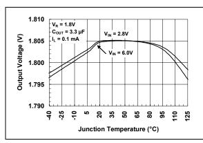
FIGURE 2-3: Output Voltage vs. Junction Temperature (0.1 mA).
