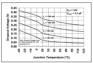
**FIGURE 2-6:** Dropout Voltage vs. Junction Temperature.
