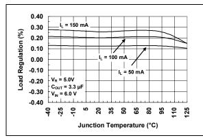
**FIGURE 2-15:** Load Regulation vs. Junction Temperature.
