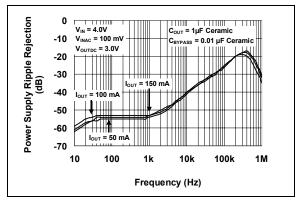
**FIGURE 2-23:** PSRR vs. Frequency  $(C_{OUT} = 1 \mu F Ceramic)$ .
