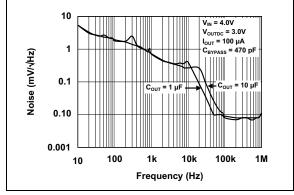
FIGURE 2-26: Output Noise vs. Frequency.
