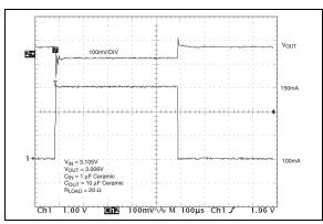
**FIGURE 2-20:** Load Transient Response in Dropout. ( $C_{OUT} = 10 \ \mu\text{F}$ ).
