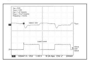
**FIGURE 2-18:** Load Transient Response.  $(C_{OUT} = 10 \ \mu\text{F})$ .
