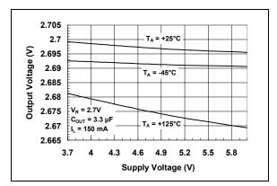
**FIGURE 2-11:** Output Voltage vs. Supply Voltage.
