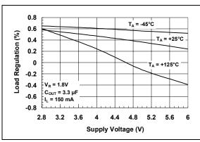
**FIGURE 2-2:** Load Regulation vs. Supply Voltage.
