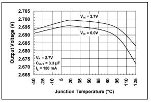
**FIGURE 2-10:** Output Voltage vs. Junction Temperature (150 mA).
