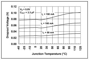
**FIGURE 2-16:** Dropout Voltage vs. Junction Temperature.
