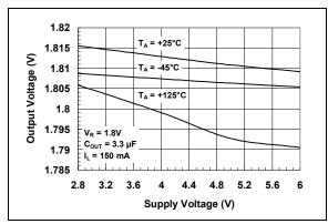
FIGURE 2-5: Output Voltage vs. Supply Voltage.
