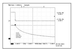
FIGURE 2-21: Shutdown Delay Time.
