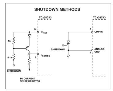
Shutdown can be accomplished by either pulling I<sub>SENSE</sub> above 1 volt or pulling CMPTR, pin 1 to GND. This will set the PWM latch so that the output will remain low until the next clock pulse after the shutdown condition is removed.
