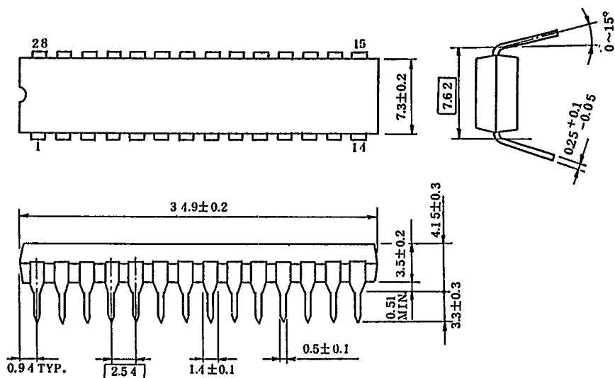
Note: Package width and length do not include mold protrusion,
