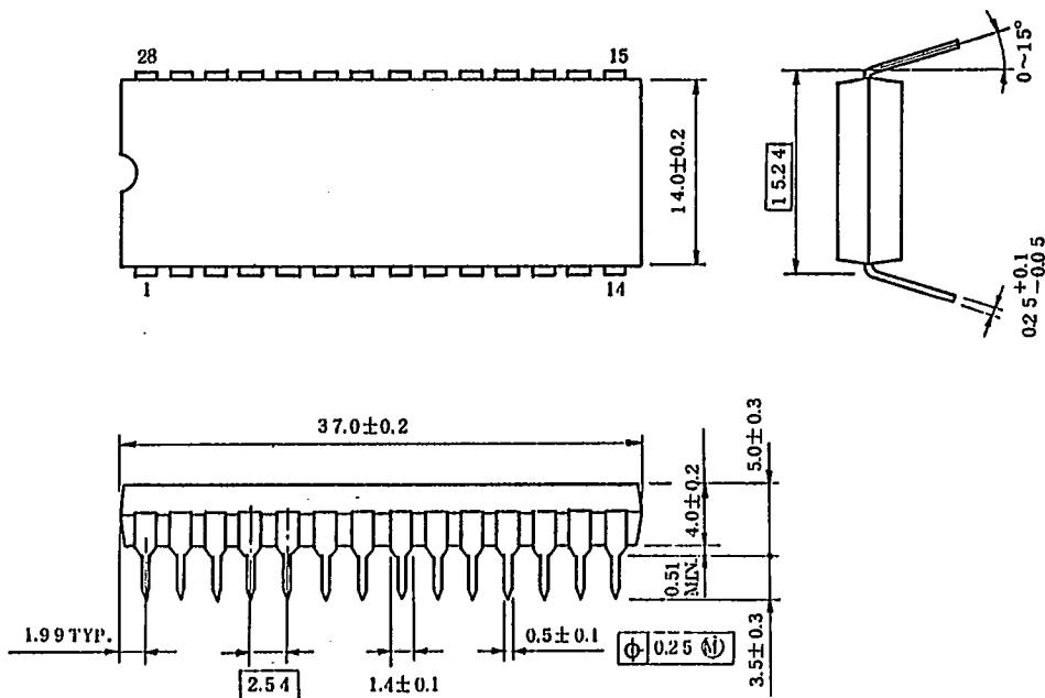
NOTES: Package width and length do not include mold protrusion,
