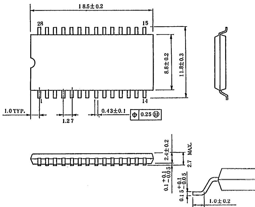
Note: Package width and length do not include mold protrusion,
