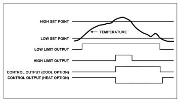
Figure 1: TC620/621 Input vs. Output Logic
