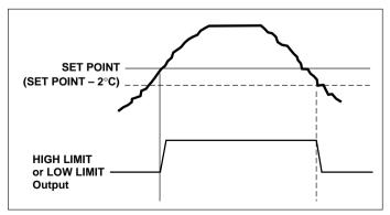
Figure 3: Built-in Hysteresis on Low Limit and High Limit Outputs
