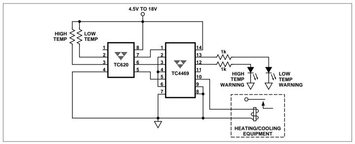
Figure 8. TC620 Heating/Cooling Application
