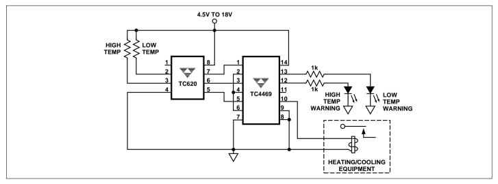
Figure 7 TC620 Heating/Cooling Application
