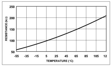
Figure 2. TC620 Sense Resistors vs. Trip Temperature
