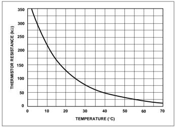
Figure 4. Typical Thermistor Resistance vs. Temperature
