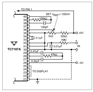
Figure 23. TC7107A Internal Reference (200mV Full-Scale, 3RPS,  $V_{\bar{I}N}$  Tied to GND for Single Ended Inputs).
