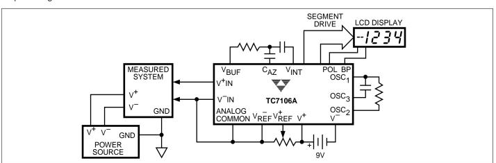
Figure 8 Common-Mode Voltage Removed in Battery Operation with  $V_{vv} = Analog Common$
