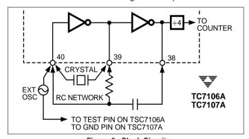
Figure 6. Clock Circuits
