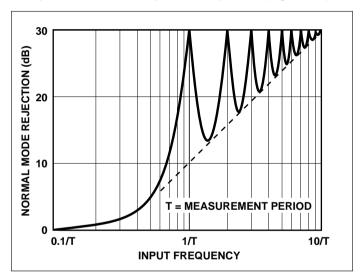
Figure 2B. Normal-Mode Rejection of Dual Slope Converter
