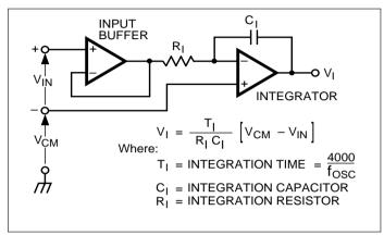
Figure 9. Common-Mode Voltage Reduces Available Integrator Swing. (V<sub>COM</sub> ≠ V<sub>IN</sub>)
