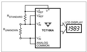
Figure 17. Low Parts Count Ratiometric Resistance
