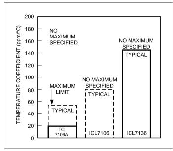
Figure 10. Analog Common Temperature Coefficient
