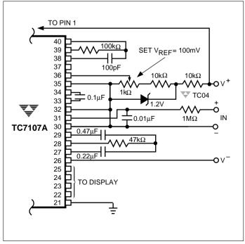
Figure 26. TC7107A With a 1.2V External Band-Gap Reference. (V<sub>IN</sub> Tied to Common.)
