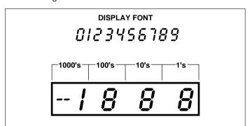
Figure 4. Display Font and Segment Assignment
