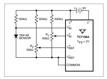
Figure 19. Temperature Sensor
