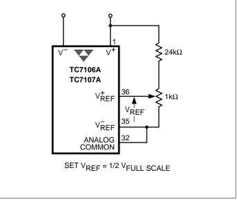
Figure 11. Internal Voltage Reference Connection
