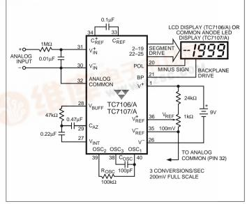
Figure 1. TC7106/A/7/A Typical Operating Circuit
