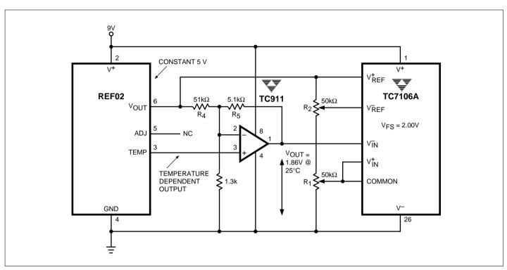
Figure 21. Integrated Circuit Temperature Sensor
