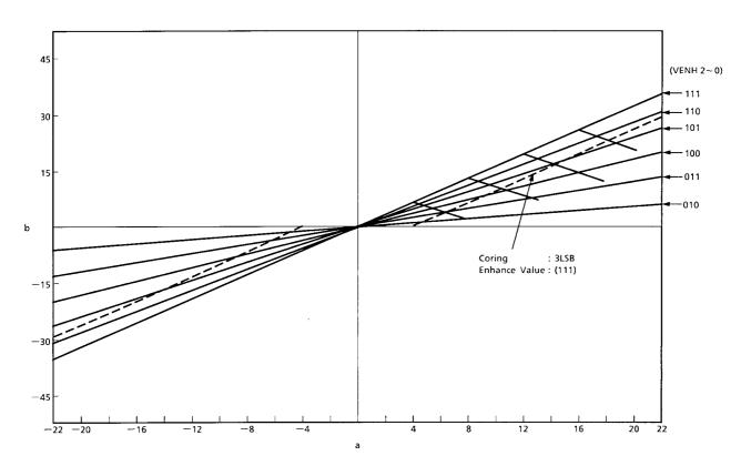
Relation between difference a in luminous signal to be enhanced during 1H and applied enhance amount b. Both a and b are LSB amounts. 1LSB  $\stackrel{\Leftarrow}{=} 0.005\,\text{V}$
