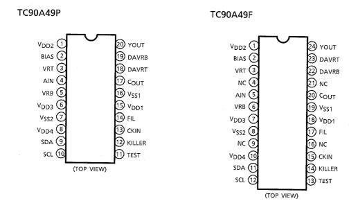
The NC which was writting in PIN ASSIGNMENT must use the open condition.
