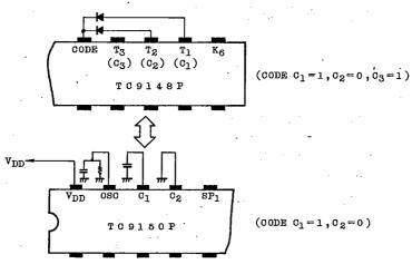
The combination of Code Bits of TC9148P and TC9150P is shown in Table 2
