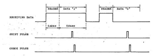
The status of receiving data, shift pulse and check pulse is shown above. Shift pulse is provided in the data center by taking frequency margins of the transmitter and the receiver into consideration.
