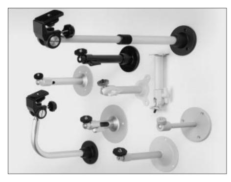
The TC9200 Series Indoor Camera Mounts can be used with CCD cameras with fixed lenses. These sturdy, attractive mounts have fully adjustable mount heads and standard 1/4-20 camera mounting bolts. Maximum load capability ranges from 2 kg (4.4 lb) to 10 kg (22 lb). These versatile models can be used as pedestal, wall, or ceiling mounts and are well suited for use with CCD cameras.
