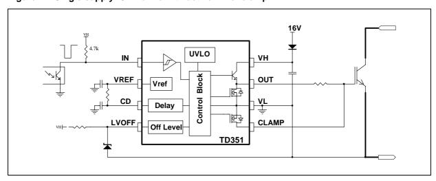
Figure 13: Use of pulse transformer signals
