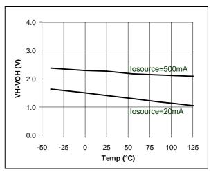
Figure 11: Source current vs temperature
