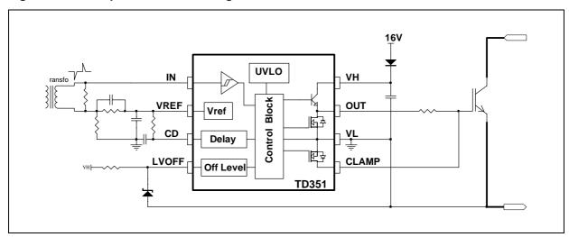
Figure 14: Large IGBT drive with negative voltage gate drive and optional current buffers
