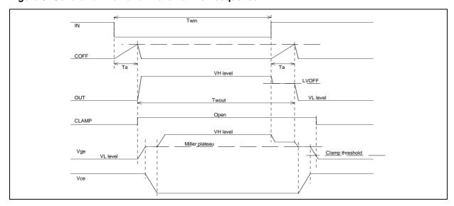
Figure 4: input and output waveform dynamic parameters
