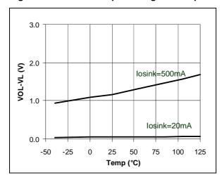
Figure 8: Sink current vs temperature
