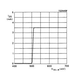
Fig.6 Keyed AGC output voltage  $I_{20}$  as a function of input voltage  $V_{14}$ . Measured in test circuit Fig.1 at  $V_3 = 2$  V;  $V_{20} = 8.5$  V.
