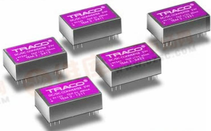
The TEM-2 series is a family of isolated dc/dc converters in a DIP-24 package. They offer tight line/ load regulation and 500 VDC I/O-isolation. Standard features include an internal filter to reduce reflected input ripple current and to guarantee low output noise. This product series provides a cost effective solution by many industrial or consumer electronics applications.
