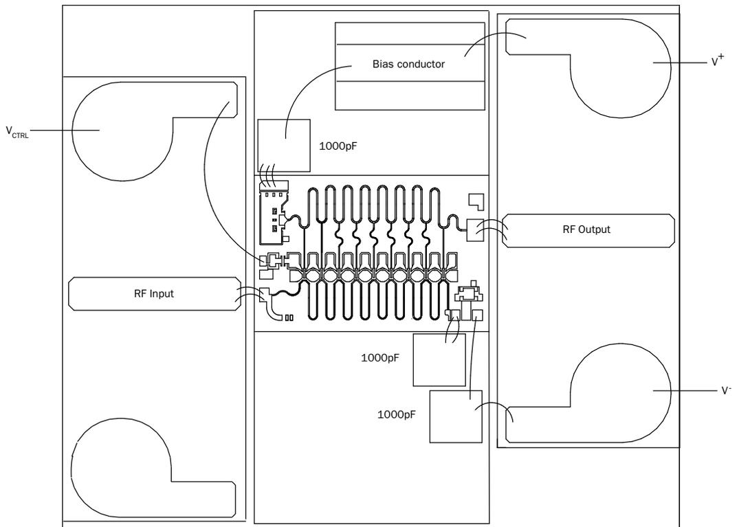
RF connections: Thermocompression bond using two 1-mil diameter, 20 to 30-mil-length gold bond wires at RF Input and at RF Output for optimum RF performance.
