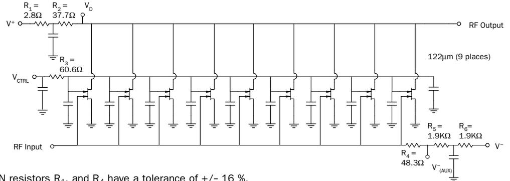
TaN resistors  $R_1$ , and  $R_4$  have a tolerance of  $\pm 16\%$ .
