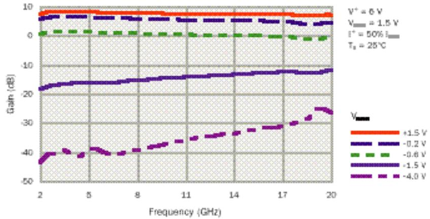
V<sub>CTRL</sub> for particular gain levels is shown for reference only and may vary from device to device.
