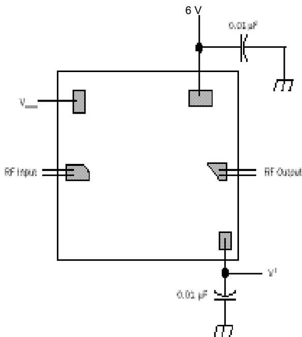
RF connections: Bond using two 1.0-mil diameter, 20-mil-length gold bond wires at both RF Input and RF Output.
