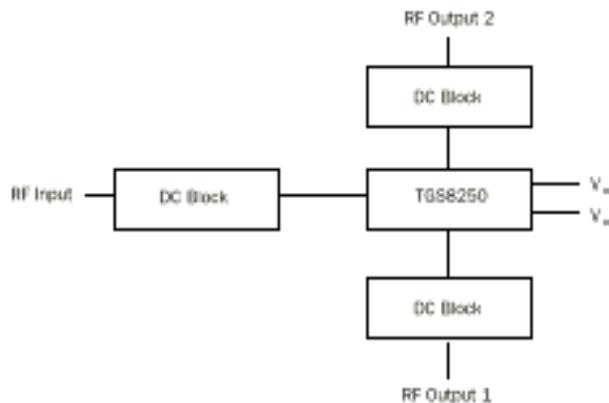
RF connections: Bond using 1-mil diameter, 20 to 25-mil length gold wire at both RF Input and RF Output ports for optimum RF performance.
