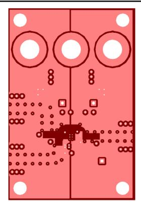
Figure 67. THS3201 EVM Board Layout (Third Layer, Power)
