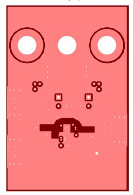
Figure 66. THS3201 EVM Board Layout (Second Layer, Ground)
