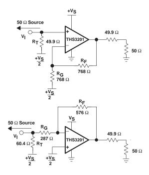
Figure 52. DC-Coupled Single Supply Operation
