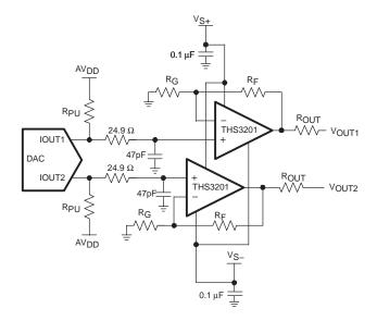
Figure 56. Differential DAC Driver Circuit
