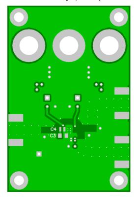
Figure 68. THS3201 EVM Board Layout (Bottom Layer)
