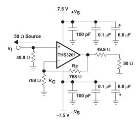
Figure 50. Wideband, Noninverting Gain Configuration
