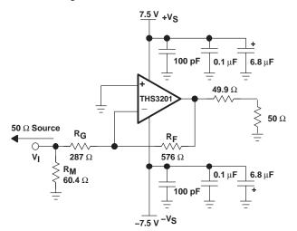
Figure 51. Wideband, Inverting Gain Configuration
