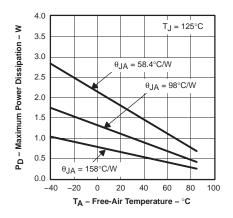
Results are With No Air Flow and PCB Size = 3"x3"  $\theta_{JA} = 58.4^{\circ}$ C/W for 8-Pin MSOP w/PowerPad (DGN)  $\theta_{JA} = 98^{\circ}$ C/W for 8-Pin SOIC High Test PCB (D)  $\theta_{JA} = 158^{\circ}$ C/W for 8-Pin MSOP w/PowerPad w/o Solder
