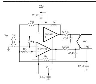
Figure 55. Differential ADC Driver Circuit 2
