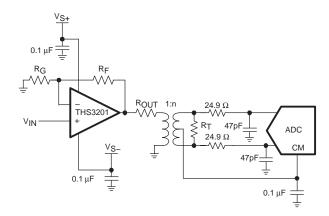
Figure 54. Differential ADC Driver Circuit 1
