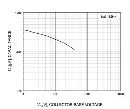
Figure 4. Collector Output Capacitance
