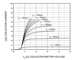
Figure 1. Static Characteristic
