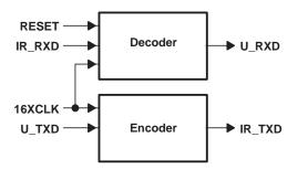
A transceiver device is needed to interface to the photo-sensitive diode (PIN) and the light emitting diode (LED). A UART is needed to interface to the serial data lines.
