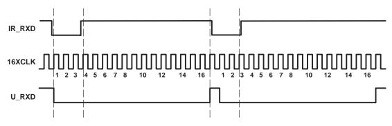
Figure 6. Timing Causing 1-clock-wide Pulse Between Consecutive Ones
