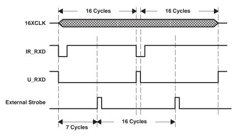
Figure 7. Recommended Strobing For Decoded Data
