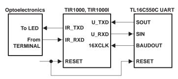
Figure 1. Typical application of the TIR1000, TIR1000I
