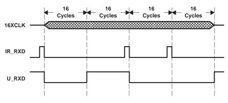
Figure 9. Positive IR\_RXD Pulse Decode – Macro View
