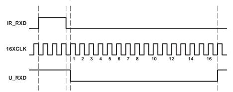
Figure 8. Positive IR\_RXD Pulse Decode – Detailed View
