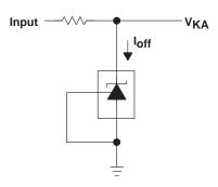
Figure 3. Test Circuit for I<sub>off</sub>
