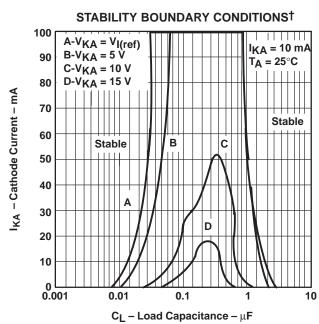
$^{\dagger}$  The areas under the curves represent conditions that may cause the device to oscillate. For curves B, C, and D, R2 and V+ are adjusted to establish the initial V<sub>KA</sub> and I<sub>KA</sub> conditions with C<sub>L</sub> = 0. V<sub>BATT</sub> and C<sub>L</sub> are then adjusted to determine the ranges of stability.
