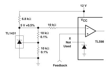
Figure 24. PWM Converter With 0.5% Reference
