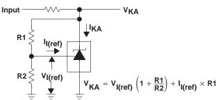
Figure 2. Test Circuit for  $V_{(KA)} > V_{ref}$
