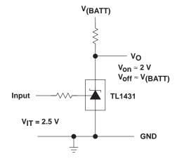
Figure 17. Single-Supply Comparator With Temperature-Compensated Threshold
