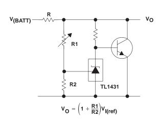
Figure 20. Higher-Current Shunt Regulator
