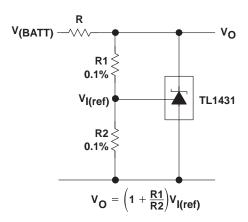
NOTE A: R should provide cathode current  $\geq$ 1 mA to the TL1431 at minimum  $V_{(BATT)}$ .
