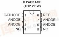
NC – No internal connection ANODE terminals are connected internally.
