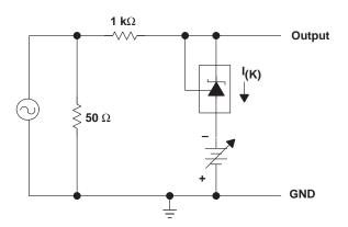
TEST CIRCUIT FOR REFERENCE IMPEDANCE
