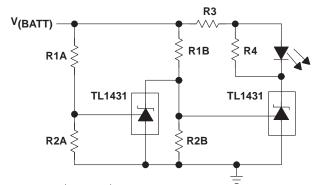
$$\begin{aligned} & \text{Low Limit} = \left(1 + \frac{R1B}{R2B}\right) V_{\text{I(ref)}} & & \text{LED on When} \\ & \text{High Limit} = \left(1 + \frac{R1A}{R2A}\right) V_{\text{I(ref)}} & & \text{Low Limit} < V_{\text{(BATT)}} < \text{High Limit} \end{aligned}$$
