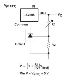
Figure 19. Output Control of a Three-Terminal Fixed Regulator
