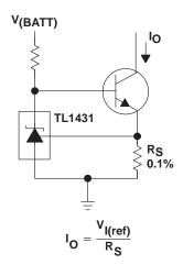
Figure 28. Precision Constant-Current Sink
