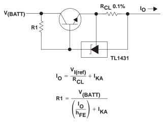
Figure 27. Precision Current Limiter
