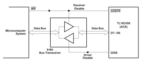
Figure 8. Typical Interface for a High-Capacity Data Bus
