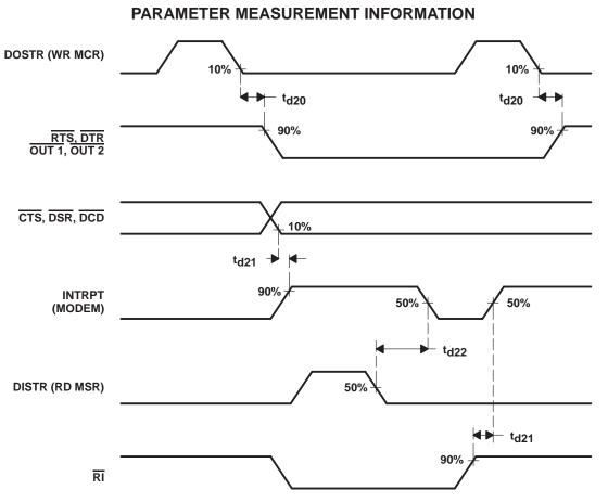
Figure 6. Modem Control Timing Waveforms
