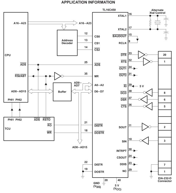
Figure 9. Typical TL16C450 Connection to a CPU
