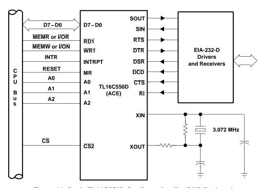
Figure 21. Basic TL16C550D Configuration (for RHB Package)
