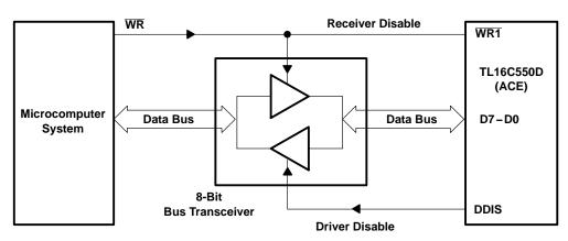
Figure 22. Typical Interface for a High Capacity Data Bus
