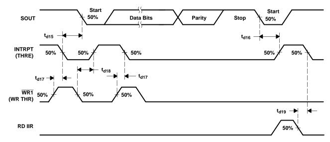
**Figure 13. Transmitter Timing Waveforms**
