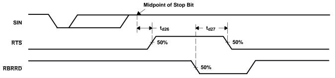
Figure 18. Auto-RTS Timing for RCV Threshold of 1, 4, or 8 Waveforms
