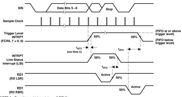
NOTE A: For a time-out interrupt,  $t_{d13} = 9$  RCLKs.
