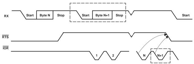
NOTES: A. N = receiver FIFO trigger level
