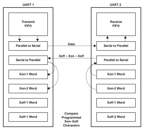
Figure 4. Software Flow Control Example
