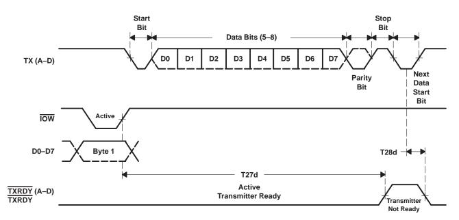
Figure 20. Transmit Ready Timing in None FIFO Mode
