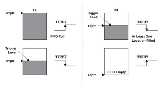
Figure 8. TXRDY and RXRDY in DMA Mode 1
