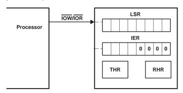
Figure 6. FIFO Polled Mode Operation
