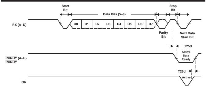
Figure 17. Receive Ready Timing in None FIFO Mode
