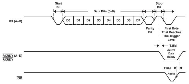
Figure 18. Receive Timing in FIFO Mode
