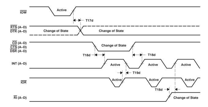
Figure 15. Modem Input/Output Timing
