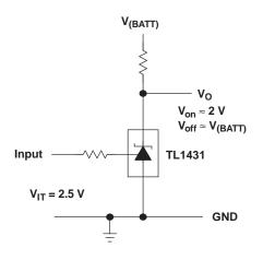
Figure 17. Single-Supply Comparator With Temperature-Compensated Threshold
