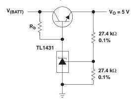
NOTE A:  $R_b$  should provide cathode current  $\geq 1$  mA to the TL1431.
