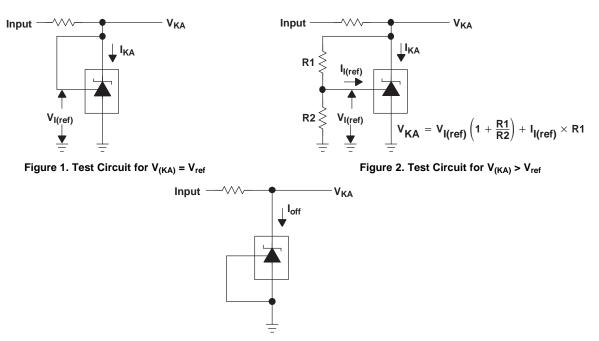
Figure 3. Test Circuit for Ioff
