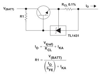
Figure 27. Precision Current Limiter
