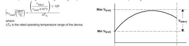
$\alpha_{V_{l(ref)}}$  is positive or negative, depending on whether minimum  $V_{l(ref)}$  or maximum  $V_{l(ref)}$ , respectively, occurs at the lower temperature.
