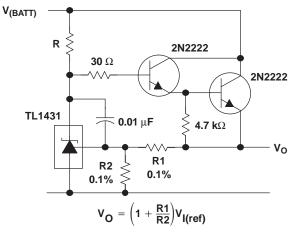
NOTE A: R should provide cathode current ≥1 mA to the TL1431 at minimum V<sub>(BATT)</sub>.
