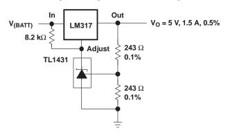
Figure 22. Precision 5-V, 1.5-A, 0.5% Regulator
