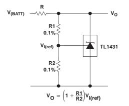
NOTE A: R should provide cathode current  $\geq$ 1 mA to the TL1431 at minimum V<sub>(BATT)</sub>.
