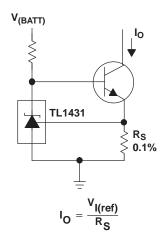
Figure 28. Precision Constant-Current Sink
