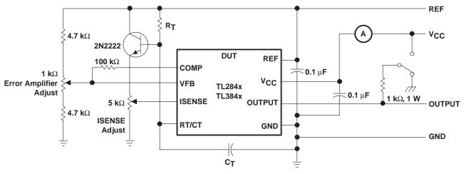
Figure 6. Open-Loop Laboratory Test Fixture
