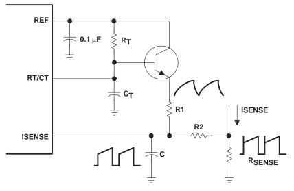
Figure 8. Slope Compensation
