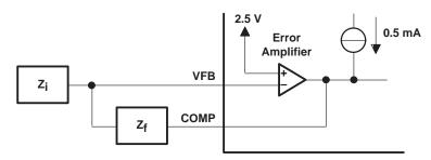
NOTE A: Error amplifier can source or sink up to 0.5 mA.
