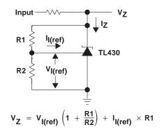
Figure 2. Test Circuit for  $V_Z > V_{I(ref)}$
