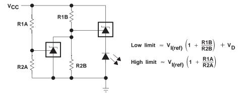
Figure 11. V<sub>CC</sub> Monitor
