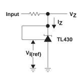
Figure 1. Test Circuit for  $V_Z = V_{I(ref)}$
