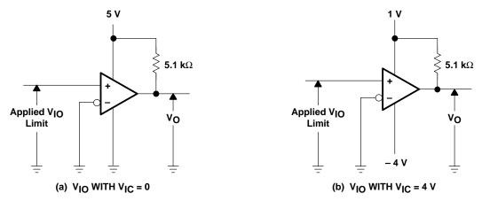
Figure 1. Method for Verifying That Input Offset Voltage Is Within Specified Limits
