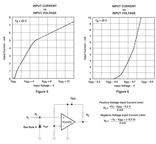
NOTE A: If the correct output state is required when the negative input exceeds VSS, a schottky clamp is required.
