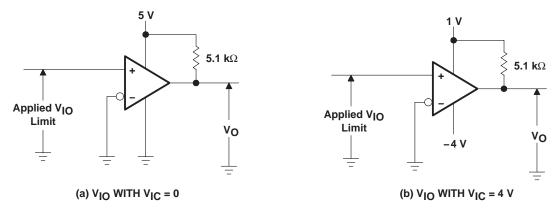
Figure 1. Method for Verifying That Input Offset Voltage is Within Specified Limits
