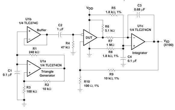
Figure 2. Circuit for Input Offset Voltage Measurement
