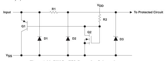
Figure 4. LinCMOS™ ESD-Protection Schematic
