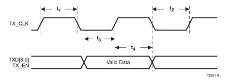
Figure 7-4. 100Mb/s MII Transmit Timing
