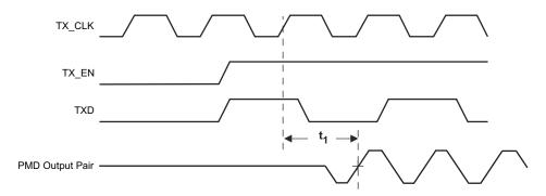
Figure 7-13. 10BASE-T Transmit Timing (Start of Packet)
