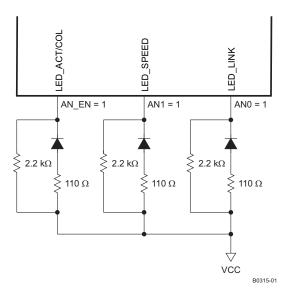
Figure 3-2. AN Pin Configuration and LED Loading Example
