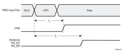
Figure 7-9. 100BASE-TX Receive Packet Latency Timing
