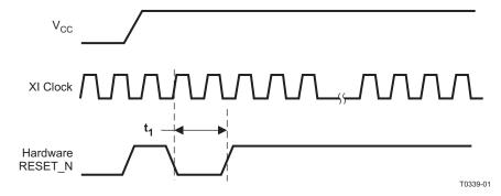
Figure 7-2. Reset Timing
