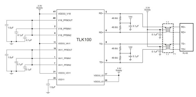
Figure 2-1. Power Scheme for Single Supply Operation
