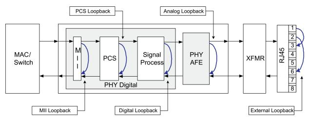
Figure 3-3. Block Diagram, Near-End Loopback Mode
