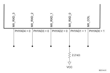
Figure 3-1. PHYAD Configuration Example
