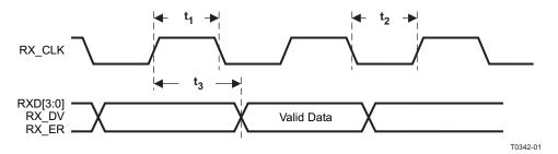
Figure 7-5. 100Mb/s MII Receive Timing
