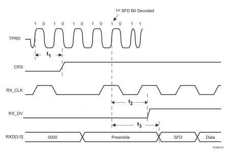
Figure 7-15. 10BASE-T Receive Timing (Start of Packet)
