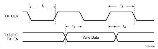
Figure 7-11. 10 Mb/s MII Transmit Timing
