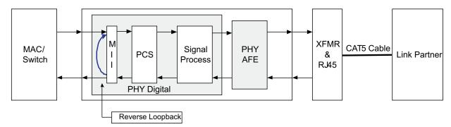
Figure 3-4. Block Diagram, Far-End Loopback Mode
