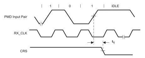
Figure 7-16. 10BASE-T Receive Timing (End of Packet)
