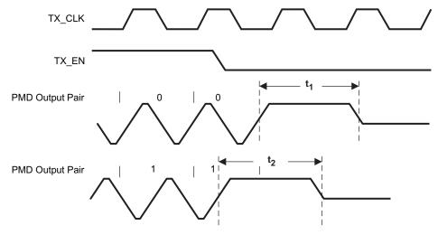
Figure 7-14. 10BASE-T Transmit Timing (End of Packet)
