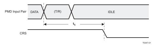
Figure 7-10. 100BASE-TX Receive Packet Deassertion Timing
