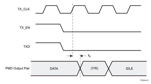
Figure 7-7. 100BASE-TX Transmit Packet Latency Timing
