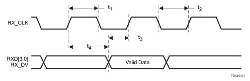
Figure 7-12. 10Mb/s MII Receive Timing
