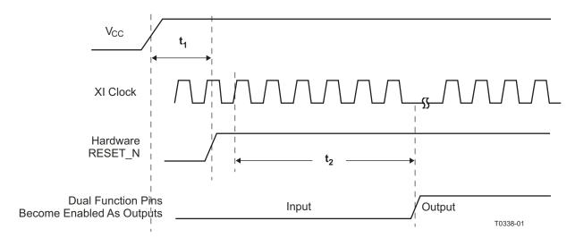
Figure 7-1. Power Up Timing
