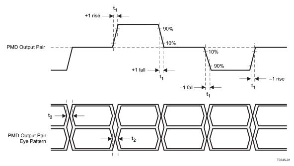
Figure 7-8. 100BASE-TX Transmit Timing (t<sub>R/F</sub> and Jitter)
