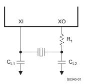
Figure 5-2. Crystal Oscillator Circuit
