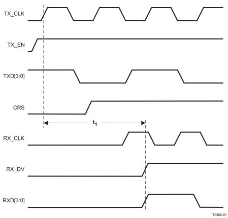
NOTE: Measurement is made from the first rising edge of TX\_CLK after assertion of TX\_EN.
