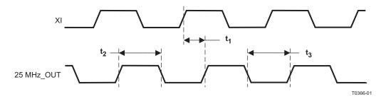
Figure 7-24. 25 MHz\_OUT Timing
