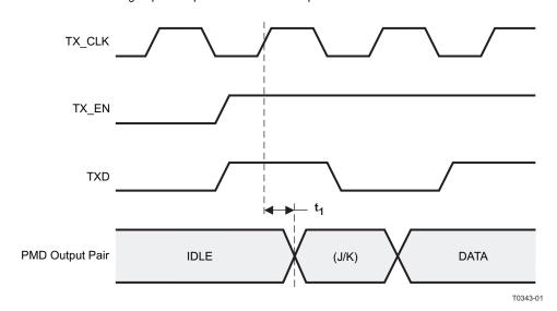
Figure 7-6. 100BASE-TX Transmit Packet Latency Timing
