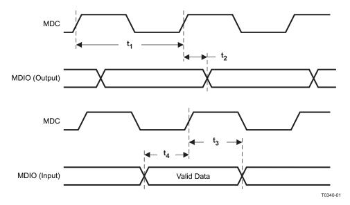
Figure 7-3. MII Serial Management Timing
