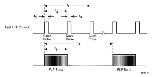
Figure 7-19. Auto-Negotiation Fast Link Pulse (FLP) Timing
