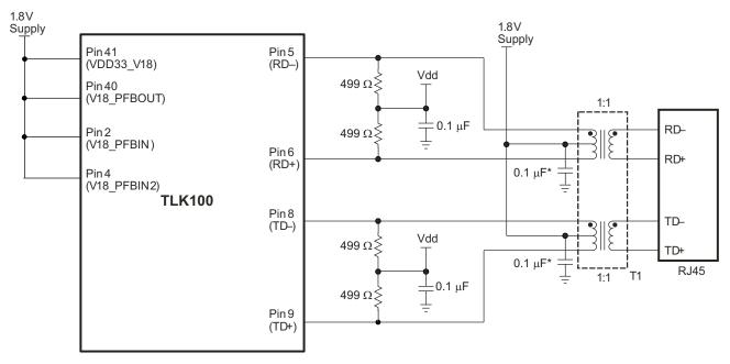
Figure 2-2. Power Scheme for Operation With External 1.8V Supply
