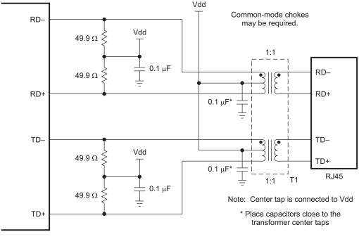
Place resistors and capacitors close to the device.
