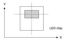
(Note 2): Luminous radiation output effective angle = ±25 degree
