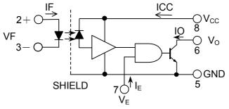
A  $0.1\mu F$  bypass capacitor must be connected Between pins 8 and 5.(See Note 1)
