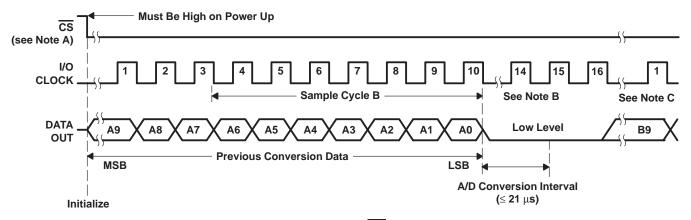
Figure 11. Timing for 16-Clock Transfer Not Using CS (Serial Transfer Completed After 21 μs)
