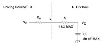
V<sub>I</sub> = Input Voltage at ANALOG IN
