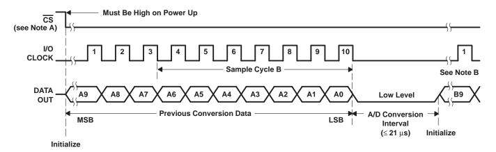
Figure 7. Timing for 10-Clock Transfer Not Using CS
