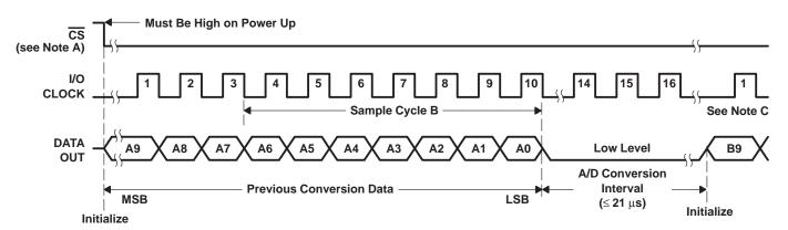
Figure 9. Timing for 16-Clock Transfer Not Using CS (Serial Transfer Completed Within 21 μs)
