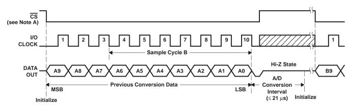
Figure 6. Timing for 10-Clock Transfer Using CS
