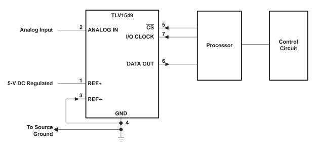
Figure 13. Typical Serial Interface
