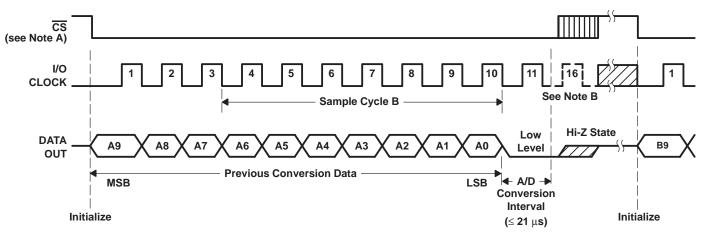
Figure 10. Timing for 11- to 16-Clock Transfer Using CS (Serial Transfer Completed After 21 μs)
