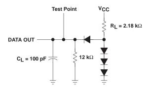
Figure 2. Load Circuit
