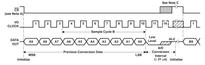
Figure 8. Timing for 11- to 16-Clock Transfer Using CS (Serial Transfer Completed Within 21 μs)
