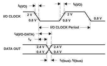
Figure 5. I/O CLOCK and DATA OUT Voltage Waveforms
