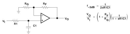
Figure 35. Single-Pole Low-Pass Filter
