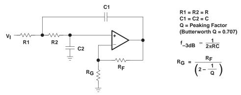
Figure 36. 2-Pole Low-Pass Sallen-Key Filter
