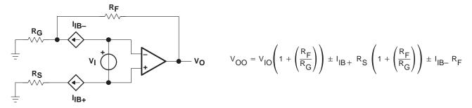
Figure 34. Output Offset Voltage Model
